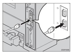
2 Connect the other end of the 1394 interface cable to the computer or the other IEEE 1394 node.
