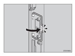
Fasten the controller board with the two screws to the printer.
