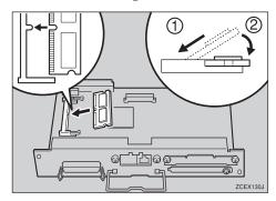
**9** Set the controller board to the "∇" position, and then slide it into the printer slowly until it stops.
