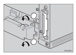
A Slowly insert the Hard Disk Drive while aligning it with the top and bottom rails in the printer, until it stops.
